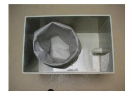
In order to carry out a flocculation, add a dose of flocculant powder in the water to be treated, allow to stir for a few minutes and once the flocs are formed, let the water pass through the filter. This operation takes about five minutes. The average dose of powder used is about 100 grams per 100 litres of water to be treated.
