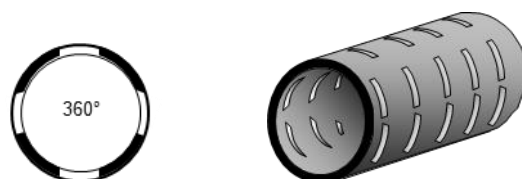
Illustration 20 – Tuyau de drainage perforé (360°)
