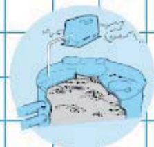
Home Aerobic Sewage Treatment System
