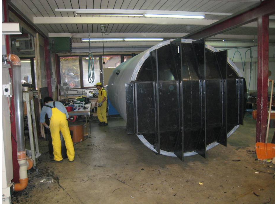
Tank with reinforced inclined base (for laying in the vicinity of the water table)
