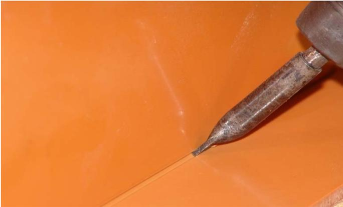
1. Tack welding is a necessary operation in order to obtain a good weld. This hot assembly operation, with no required additional material, makes it possible to plug the spaces between the elements and fix them slightly before welding them.
