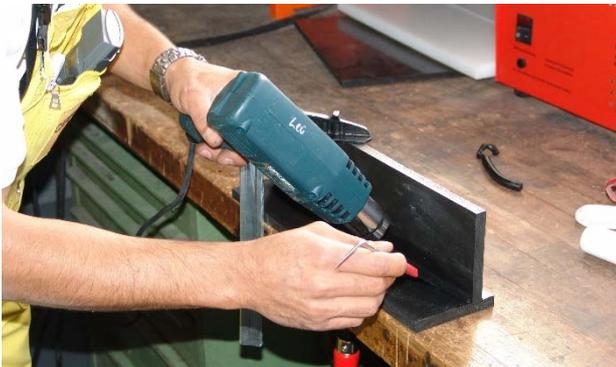
2. The welder heats the tack welded elements with a blow-dryer. His experience allows him to test the temperature of the support by pressing a metal point on the material which softens through heating.
