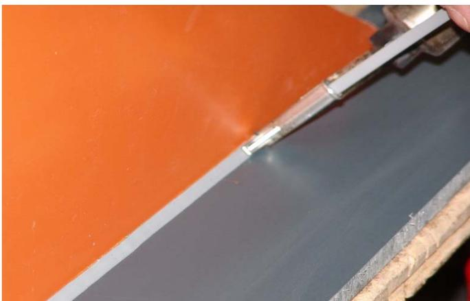
3. The pressure exerted on the rod and the welding nozzle is sufficient to obtain excellent adhesion of the welding nozzle. The orange or grey colour of the PVC does not disrupt the weld because it is the same material, simply with a different dye.
