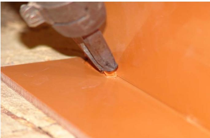
2. The welding is carried out with a suitable nozzle. The filler material is a triangular rod. The air at over 300°C produced by the device simultaneously heats the underside of the rod and the upper face of the support.
