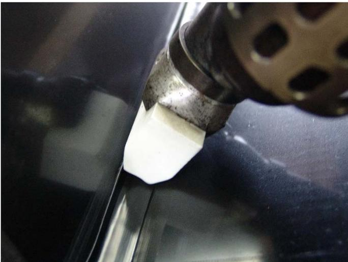
2. Tack welding, described in 'PVC welding', is necessary for both PE and PP as well as for PVC. For PE and PP, surface scraping is required before welding.
