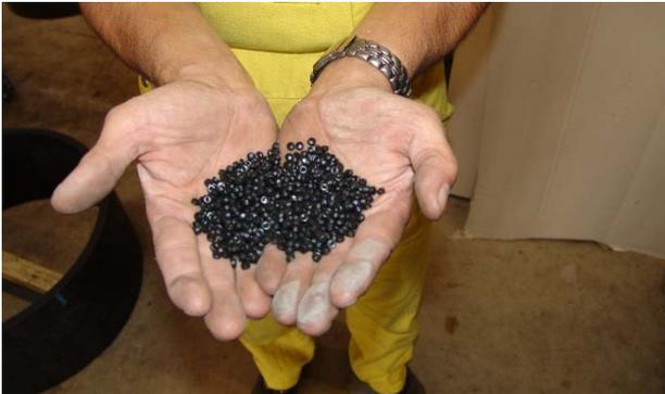
1. The raw material is in the form of granulated PE (polyethylene) which is used to fill the silo placed on the extruder.
