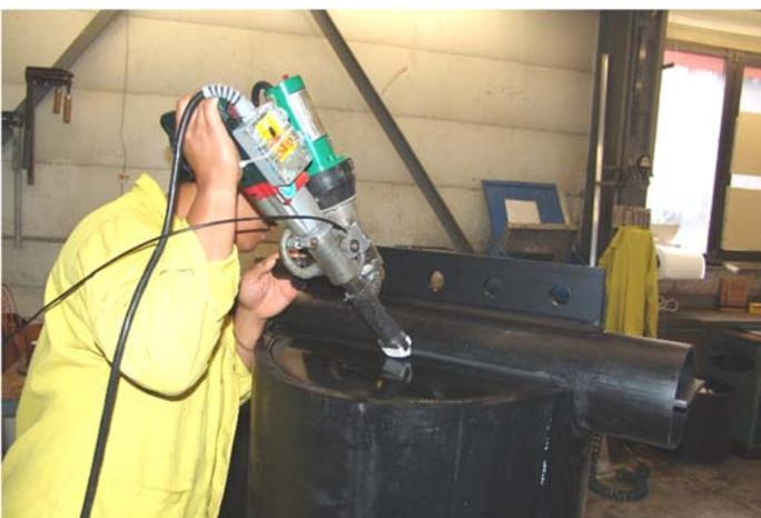
3. Welding of a PE chamber base with a gun-extruder. For welding in confined spaces, refer to « PE welding with Haering® extruder »
