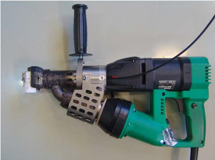
1. This gun-extruder is used for welding PE (polyethylene) and PP (polypropylene). It is fed with raw material through a wire of 4 or 5 mm in diameter. The material, heated between 200 and 220°C, is propelled through the apparatus by a worm drive.
