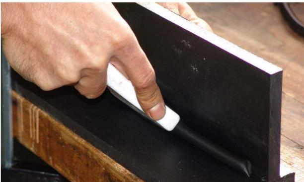
4. For all types of plastic welds, it is important that the temperature of the support and the filler material are the same and that the contact pressure is maintained. For this, we crush the weld with a Teflon spatula.
