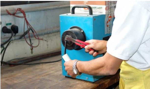
3. The extruder heats the filler material to a temperature of approximately 220°C and propels it into a sausage shape through a nozzle of variable diameter. The welder carries this weld bead inside a Teflon pipe and applies it unto the support.
