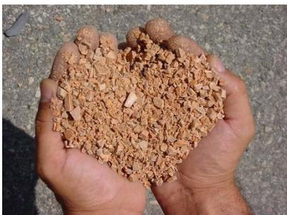
**Figure 3 :** The PVC waste is crushed by the metal knives of the crusher.
