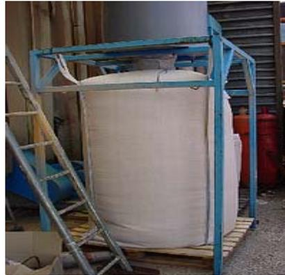
**Figure 4 :** A fan propels the crushed material into bags.
