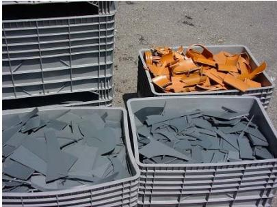
**Figure 1 :** The PVC waste is sorted by material and colour. The pipes and plates are cut into pieces.
