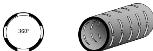
Illustration 20 – Tuyau de drainage perforé (360°)
